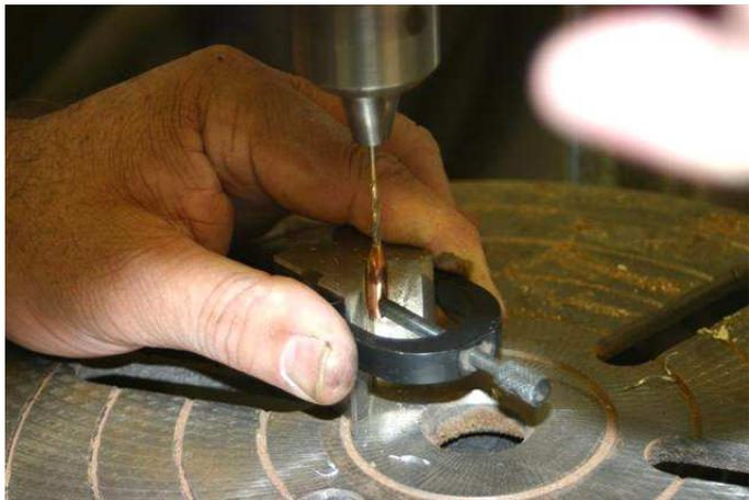
Drilling through the lead from the small end...using the hollow point hole as a guide. 5/64 bit drilled all the way through.
