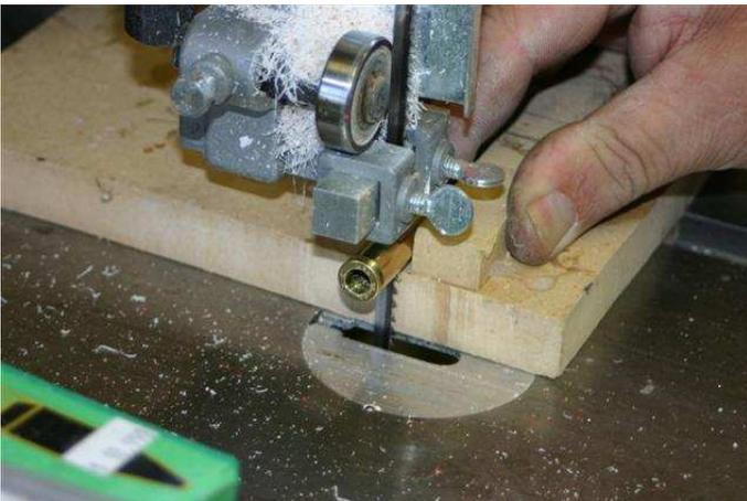
Cutting the brass on the band saw works. I use a blade that is too dull for wood. Hate to change blades so I don't use the band saw very often. However the brass is cut, some cleanup is needed to remove burrs. This will become evident as you make these pens. Just be careful..Sanding scars the brass and the scratches may not polish out.
