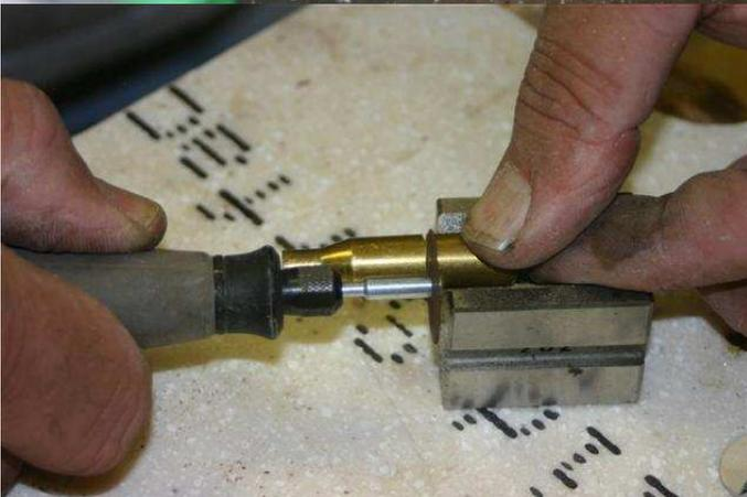
A drimmel tool with a cut-off disk can be used. Cut and turn until the brass is cut. Or, the brass can be sliced through, rotated and sliced again to finish the separation. Squaring the cut has proved to be difficult for me. Rifle brass is not a perfect cylinder which presents a squaring problem.
