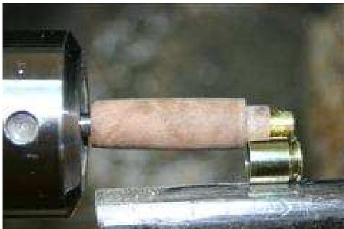
Do the same for this end as we did on the bullet end. Measure, mark and cut the tennon to fit inside the brass. Notice some of the wood has been parted off. This is necessary for the brass tube to fit flush with the flat surface on the primer end of the brass
