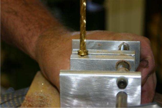
Drill out the primer end with a 5/32 bit to allow the 7mm tube to pass through and flush with the flat surface.
