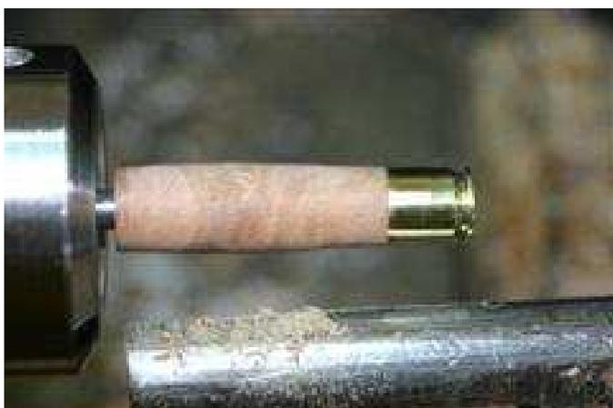
Finished tennon and fit. The two blanks are ready to mount on a mandrel and completed. Turn to desired shape, sand and finish.
