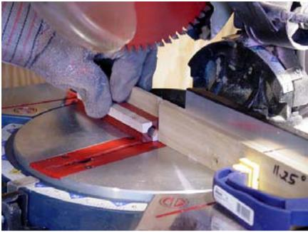
After a lot of trial and error I have finally figured out a way to use my miter saw to make very small and consistent cuts without much of a waste factor. (see figure 3) I have taken a piece wood and clamped it to each side of my saw blade. The distance between the boards where the blade drops will only allow the blade to go through the gap. This is also known as a “zero clearance fence”.
